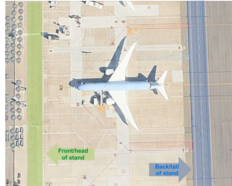
MXP Airport (Google Earth imagery) illustrating service roads located at the front and back of aircraft stands.
