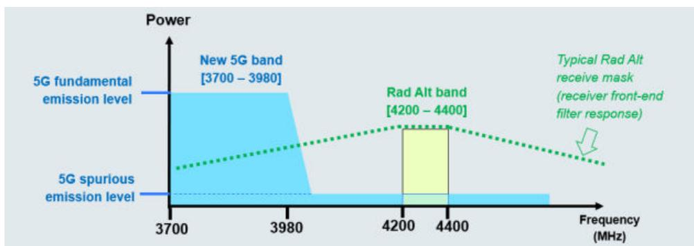
The figure above (source: *RTCA 5G Interference Report / RTCA Paper No. 274-20/PMC-2073*) shows the frequency ranges and potential for interference between radio altimeters and 5G spurious emission levels.
